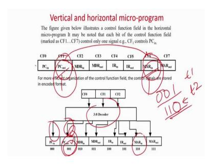
So, for example, this is one word of the control memory or this is the format of the control memory word. So,  $PC_{in}$ ,  $PC_{out}$ ,  $MDR_{in}$ ,  $MDR_{out}$  all these values are there.
